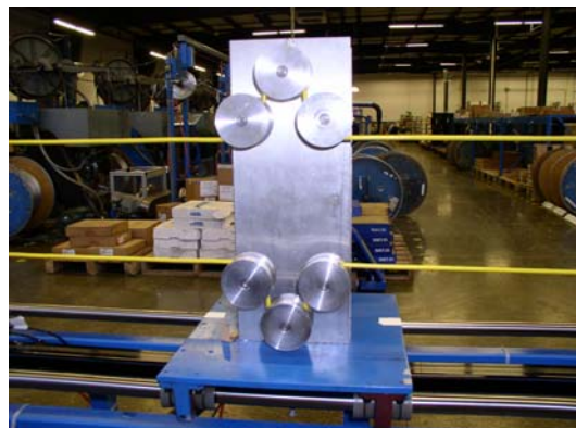
Rolling Flex Test Pulley Wrap Detail
